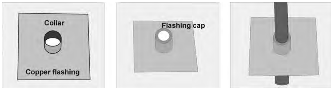
Figure 20 Copper flashing for pipe only
